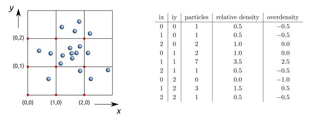
Simplified density estimation: count the particles in each cell, determine the relative density by dividing through the mean number of particles per cell (18 particles/9 cells = 2) and subtract 1 to get the overdensity (above the mean). Such overdensities along with the corresponding indizes (ix, iy, iz) can be stored in database tables.
